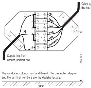
Three-phase connection 400 V system with 230 V phase against neutral conductor
